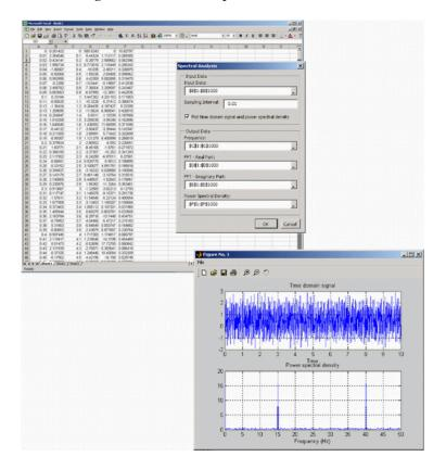
The power spectral density reveals the two signals at 15 and 40 Hz.
